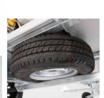
Spare wheel carrier for towing vehicle (Note tyre size)
