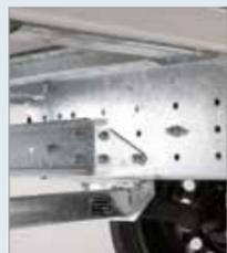
Modular frame connection to be able to extend the drawbar lengths up to 300 mm. The axle can be moved to adapt to the load
